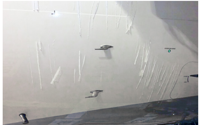
(fig.4) Example of ice ridges that remain on the lower fuselage even after completing a flight.
