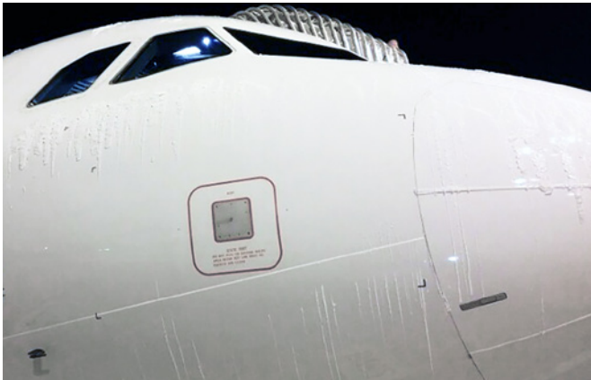
(fig.3) Example of thin ice ridges forward of the pitot probes of an A320 family aircraft
